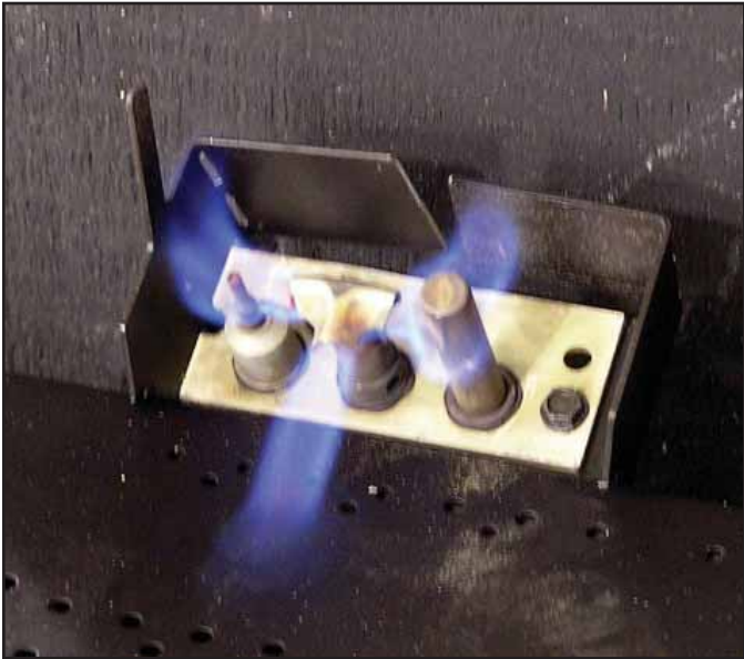
Figure 3.3 Standing Pilot Flame Patterns
